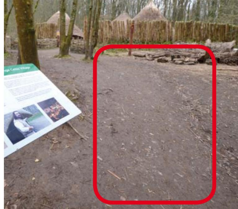
*The access route to the Village was via a bare earth pass on an uneven gradient, leading to a slip and trip hazard. The recommendation was to resurface and regrade the route in order to provide a suitable accessible surface.*
