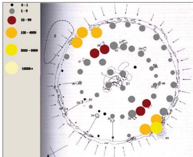
Light level survey showing values which could be obtained for “lap work” at each location (scale in lux).
